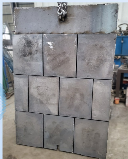
Large non-porous silo liner
